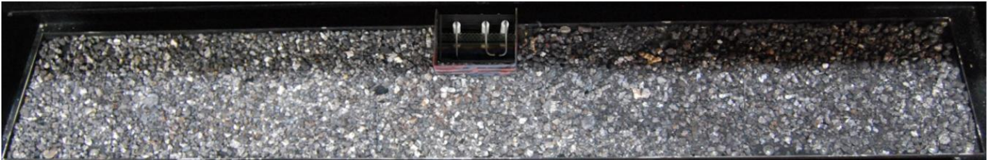
Photo 10 –Vermiculite spread on burner
